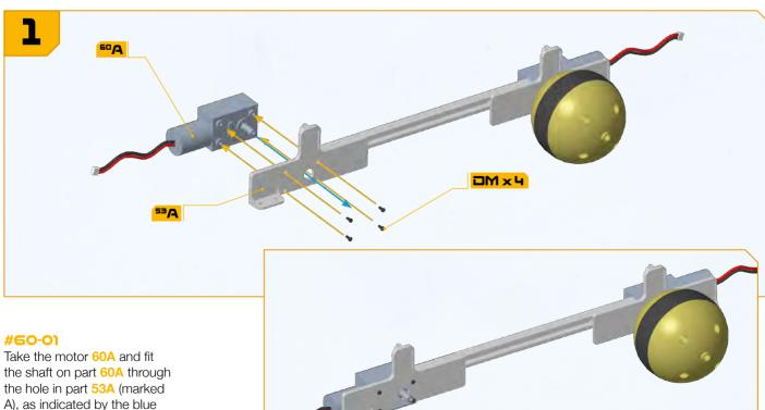
A), as indicated by the blue arrow. Fix the motor in place with four DM screws.
