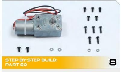
A base motor, split ring washers, two flat washers and the fixing screws.
